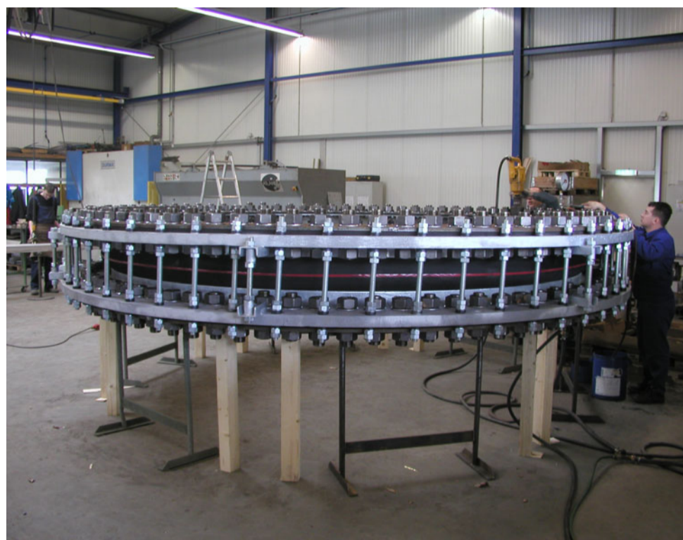
Strength test of a rubber cord expansion joint
