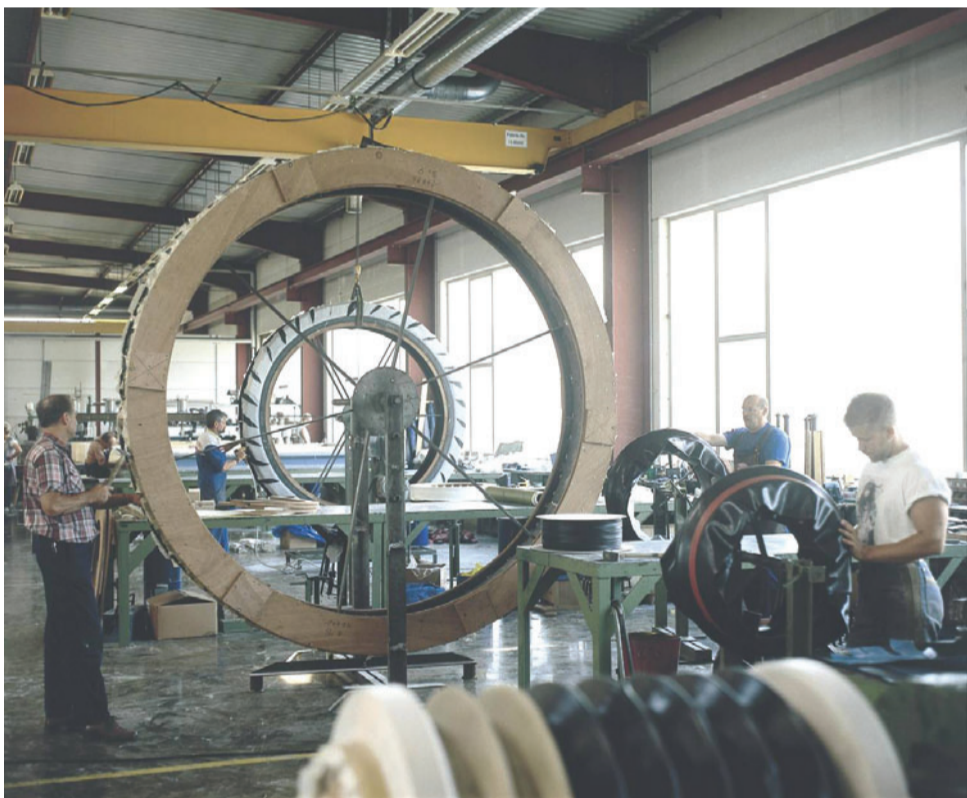
Manufacture of a rubber cord expansion joint
