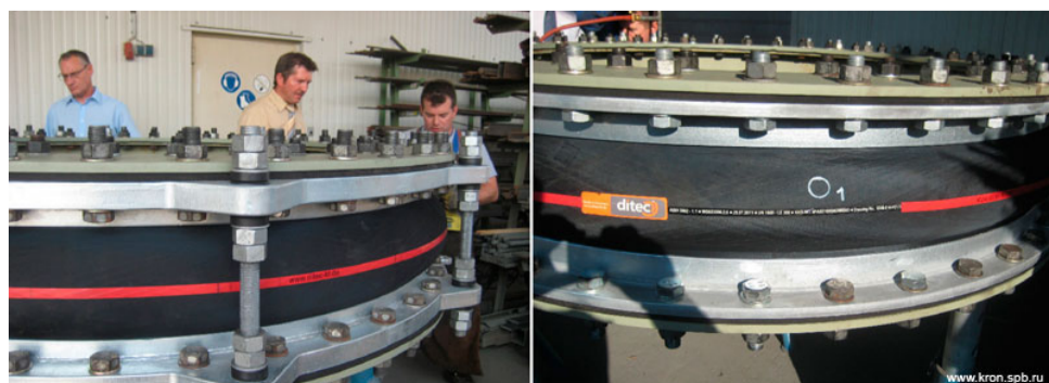
Ditec rubber cord expansion joints supplied by Kronstadt to the Beloyarskaya Nuclear Power Plant
